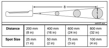
The thermometer has an 8:1 optical resolution:
